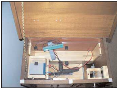
Figure 1. The OSI organ with the original MIDI removed - note the black Velcro ready to hold the new unit.
